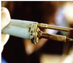
**Figure 2** On-tool extraction – soldering iron
